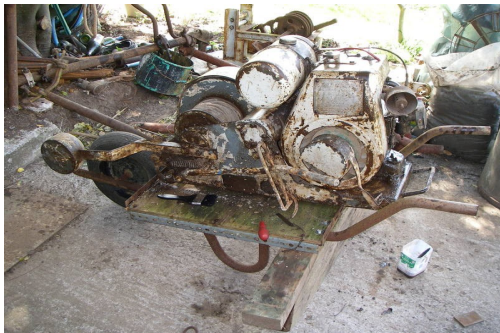
Photo 8. The Villiers hoist in need of refurbishment [Photo: T.Audsley, April 2009]
