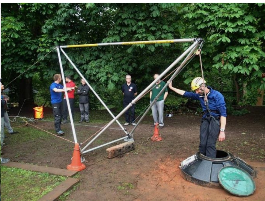
Accessing a “dangerous” pitch head using the Australian Larkin Frame. Photo by Estelle Sandford
